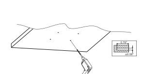
Drill pilot holes where the four marks are located with an impact drill
