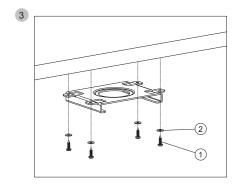
Install the mounting panel with four screws ① and four washers ②.
